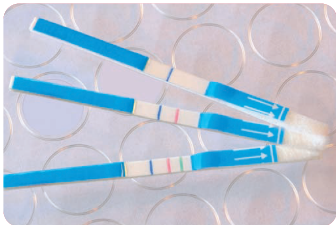
Fig. 3 Lateral flow tests using Estapor® Colored Microspheres (reference: K1-030 blue for the control, K1-030 red and K1-030 green for the analytes) and Millipore Hi-Flow™ membrane.
