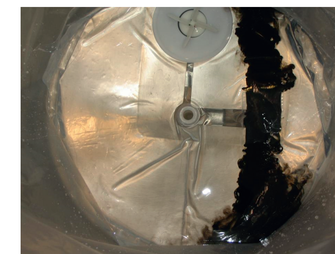
Figure 12: Retentate diverter plate directs return flow tangentially, preventing short-circuiting to the center feed port. Allowing less than 1 L
