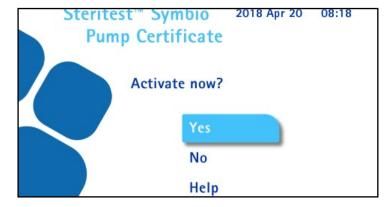
To activate the pump certificate, turn and press the control knob to select Yes.
