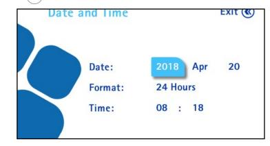
6. To set date, format, and time, turn the control knob to go from a field to another. To modify a value, push the control knob to enter the value field, turn the control knob to change the value, and press the control knob to confirm the value.
