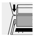
Place the **cell A** into the cell compartment.
