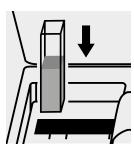
Place the cell containing the sample into the cell compartment.
