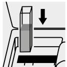
Place the cell into the cell compartment.
