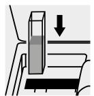
Place the cell into the cell compartment.
