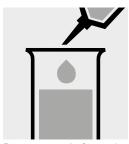
Pipette 0.5 ml of sample into a plastic vessel.
