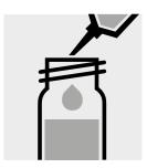
Carefully pipette 2.0 ml of the sample into a reaction cell, close tightly with the screw cap, and mix vigorously.
