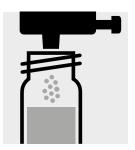
Add 1 dose of **CN-1K** using the green dosemetering cap, close the cell with the screw cap.
