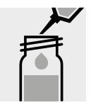
Pipette 0.20 ml of the sample into a reaction cell, close with the screw cap, and mix.
