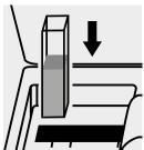
Place the cell into the cell compartment.
