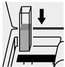
Place the cell into the cell compartment.
