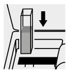
Place the cell into the cell compartment.
