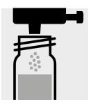
Add 1 dose of CN-1 using the green dosemetering cap, close the cell with the screw cap.
