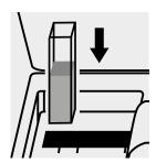
Place the cell into the cell compartment.
