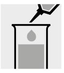
Add 1.5 ml of reagent 2 with pipette and mix.
