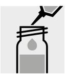
Add 1.0 ml of **B-1** with pipette, close with the screw cap, and mix.
