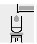
Filter the sample through a suitable filter (e.g. glass-fibre filter).
