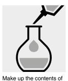
the volumetric flask to the mark with distilled water (Water for analysis EMSURE®, Cat.No. 1.16754, is recommended) and mix thoroughly.
