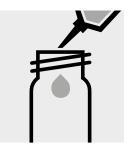
Add 9.0 ml of distilled water (Water for analysis EMSURE®, Cat.No. 1.16754, is recommended) with pipette.
