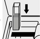
Place the cell into the cell compartment.
