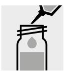
Add 0.20 ml of reagent 2 with pipette, close the cell with the screw cap, and mix.
