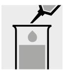
Pipette 1.0 ml of Cd-1 into a test tube.
