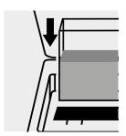
Place the cell into the cell compartment.
