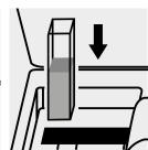
Place the cell into the cell compartment.
