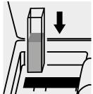
Place the cell into the cell compartment.
