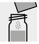
Add 1 powder pack of Molybdenum HR3 and close with the screw cap.
