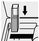
Place the cell into the cell compartment.
