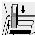
Place the cell into the cell compartment.
