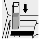
Place the cell into the cell compartment.
