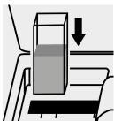
Place the cell into the cell compartment.
