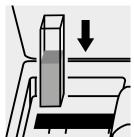
Place the cell into the cell compartment.
