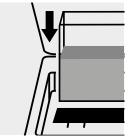
Place the cell into the cell compartment.
