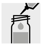
Pipette 5.0 ml of the sample into a reaction cell, do not mix!
