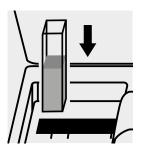
Place the cell into the cell compartment.
