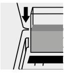
Place the cell into the cell compartment.
