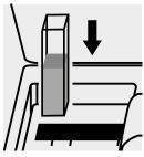
Place the cell into the cell compartment.
