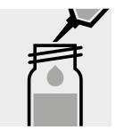
Add 0.25 ml of **Cl-1K** with pipette, close with the screw cap, and mix.
