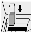
Place the cell into the cell compartment.
