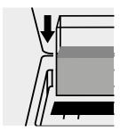
Place the blank cell into the cell compartment.
