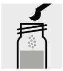
Add 1 level blue microspoon of **F-1K** to each cell, close with the screw cap.
