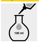
Place 50 ml of distilled water (Water for analysis acid 1 mol/l. EMSURE®, Cat.No. 1.16754, is recommended) into a 100-ml volumetric flask.
