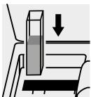
Place the cell into the cell compartment.
