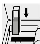
Place the cell into the cell compartment.
