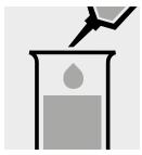
Pipette 2.0 ml of F-1 into Add 5.0 ml of water and 0.5 ml of the sample with pipette and mix.
