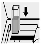
Place the cell into the cell compartment. The blank measurement is performed automatically.
