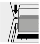
Place the cell into the cell compartment.
