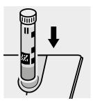
Place the **cell B** into the cell compartment. Align the mark on the cell with that on the photometer. The measurement is performed automatically.
