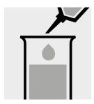
Add 1.0 ml of reagent 1 with pipette and mix.
