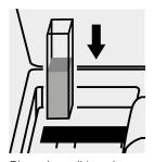
Place the cell into the cell compartment. The blank measurement is performed automatically.
