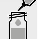
Add 2.0 ml of ethylene glycol monomethyl ether, close the test tube with the screw cap, and mix.
