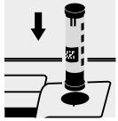
Select method with AutoSelector measuring range 5 - 160 mg/l Ca.
