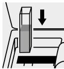
Place the cell into the cell compartment.
