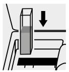
Place the cell into the cell compartment.
