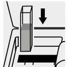
Place the cell into the cell compartment.
