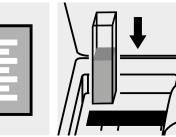
Place the cell into the cell compartment.
