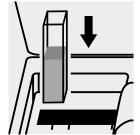
Place the cell into the cell compartment. The measurement is performed automatically.
