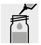
Add 1.0 ml of **reagent 1** with pipette, close the cell with the screw cap, and mix.
