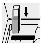
Place the cell into the cell compartment.
