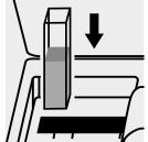
Place the cell into the cell compartment.
