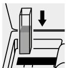
Place the cell into the cell compartment.
