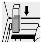
Place the cell into the cell compartment.
