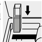
Place the cell into the cell compartment.
