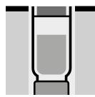
Heat the cell, standing on its head, at 120 °C in the thermoreactor for 2 hours.
