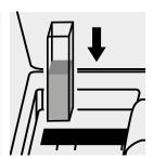
Place the cell into the cell compartment.
