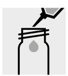
Pipette 5.0 ml of **NO<sub>3</sub>-1** into a dry empty round cell (Empty cells, Cat. No. 1.14724).
