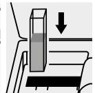
Place the cell into the cell compartment.
