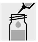
Add 0.50 ml of **Ca-2K** with pipette, close the cell with the screw cap, and mix.
