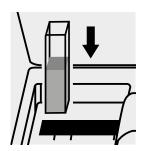
Place the cell into the cell compartment.
