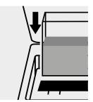
Place the cell into the cell compartment.
