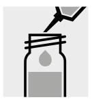
Add 6.0 ml of Au-4 with pipette, close with the screw cap.
