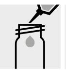
Pipette 5.0 ml of the 1:500 dilute sample into an empty round cell (Empty cells, Cat. No. 1.14724).
