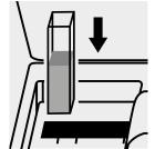
Place the cell into the cell compartment.
