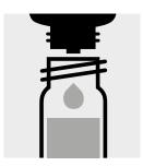
Add 6 drops of K-1K, close the cell with the screw cap, and mix.
