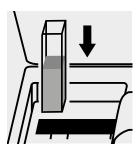
Place the cell into the cell compartment.
