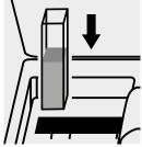
Place the cell into the cell compartment.
