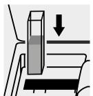
Place the cell into the cell compartment.
