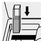
Place the cell into the cell compartment.
