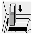
Place the cell into the cell compartment.
