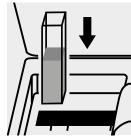
Place the cell into the cell compartment.
