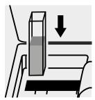
Place the cell into the cell compartment.
