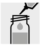
Add 5.0 ml of the sample with pipette, close with the screw cap.
