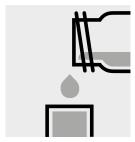
Transfer the solution into a 50-mm cell.
