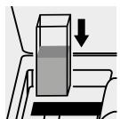
Place the cell into the cell compartment.
