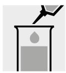
Pipette 1.0 ml of distilled water (Water for analysis EMSURE®, Cat.No. 1.16754, is recommended) into a plastic vessel.
