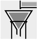
Filter the entire mixture over a hydrophobic filter acc. to ÉN 1141 [1] or §64 LFGB 31.00-7 [2]: measurement sample.
