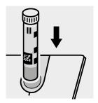
Place the cell without re-shaking into the cell compartment. Align the mark on the cell with that on the photometer.
