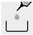
Pipette 25.0 ml of sample into a platinum dish and incinerate acc. to EN 1136 [3].
