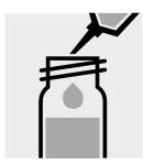
Pipette 2.0 ml of the sample into a reaction cell, **do not mix**.
