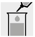
Pipette 5.0 ml of distilled water (Water for analysis EMSURE®, Cat.No. 1.16754, is recommended) into a second test tube.
