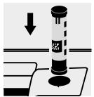
Select method with AutoSelector measuring range 5 – 150 mg/l NH<sub>4</sub>-N.
