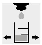
Check the chloride content of the depleted sample using MQuant® Chloride Test (Cat. No. 1.11132) according to the application (see the website): Specified value <2000 mg/l Cl<sup>-</sup>.
