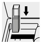
Place the cell into the cell compartment.
