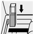
Place the cell into the cell compartment.
