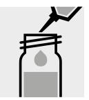
Add 0.20 ml of **Cd-1K** with pipette, close the cell with the screw cap, and mix.
