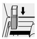
Place the cell into the cell compartment.
