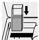
Place the cell into the cell compartment.
