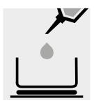
Weigh sample, accurately weighed to 1 mg, into a suitable vessel and perform a wet digestion or incinerate acc. to §64 LFGB 01.00-92 [1].
