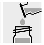
Fill the solution into a round cell.
