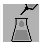
Acidify a portion of the extract with hydrochloric acid 1 mol/l Titripur® (Cat. No. 1.09057) (50 µl per 5 ml of extract).
