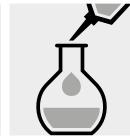
Make up the contents of the volumetric flask to the mark with distilled water (Water for analysis EMSURE®, Cat.No. 1.16754, is recommended) and mix thoroughly.
