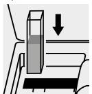
Place the cell into the cell compartment.
