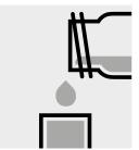
Transfer the solution into a rectangular cell.
