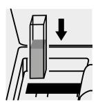
Place the cell into the cell compartment.
