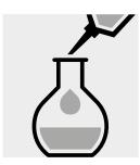
Make up the contents of the volumetric flask to the mark with distilled water (Water for analysis EMSURE®, Cat.No. 1.16754, is recommended) and mix thoroughly.
