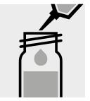
Pipette 5.0 ml of distilled Reaction time: water (Water for analysis EMSURE®, Cat.No. 1.16754, is recommended) into a second reaction cell, close with the screw cap, and mix. (Blank)
