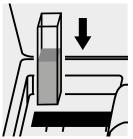
Place the cell into the cell compartment. The measurement is performed automatically.
