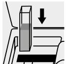
Place the cell into the cell compartment.
