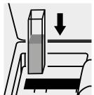
Place the cell into the cell compartment.
