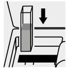
Place the cell into the cell compartment.
