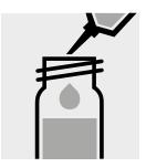
**Immediately** add 1.5 ml of **NO**<sub>3</sub>**-2** with pipette.
