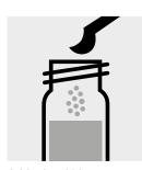
Add 1 level blue microspoon of CN-4, close the cell with the screw cap
