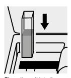
Place the cell into the cell compartment.
