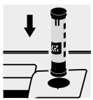
Select method with AutoSelector measuring range 0.002 - 0.100 mg/l.
