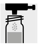
Add 1 dose of P-2K using the blue dosemetering cap, close the cell with the screw cap.
