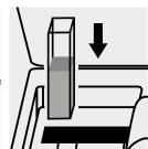
Place the cell into the cell compartment.
