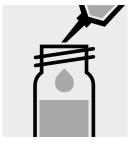
Add 10 ml of n-butyl acetate and close the test tube with the screw сар.
