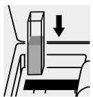
Place the cell into the cell compartment.
