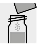
Add 1 powder pack of Molybdenum HR1, close with the screw cap, and dissolve the solid substance.
