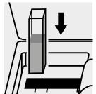
Place the cell into the cell compartment.
