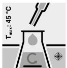
Add slowly to each Erlenmeyer flask 25 ml of Sulfuric acid for the determination of COD (Cat. No. 1.17048) with glass pipette under cooling and stirring.
