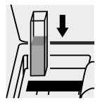
Place the cell into the cell compartment.
