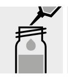
Add 1.0 ml of **reagent 1** with pipette, close the cell with the screw cap, and mix.
