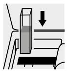
Place the cell into the cell compartment.
