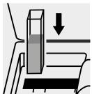
Place the cell into the cell compartment.
