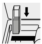
Place the cell into the cell compartment.
