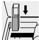
Place the cell into the cell compartment.
