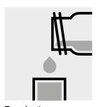
Transfer the measurement sample into the cell and measure **immediately**.
