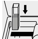
Place the cell into the cell compartment.
