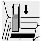
Place the cell into the cell compartment.
