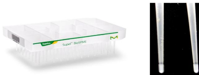
**Figure 2.** (left) Supel™ BioSPME device. (right) close-up of two pins to show the C18 coating of 2 mm on the outside of the pin.
