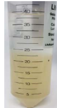
Figure B. LifeSupport™ compacted at the bottom of the centrifuge tube with liquid supernatant on top.
