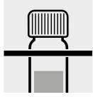
Replace the cell in the rack for complete cooling to room temperature. **Very important!**
