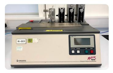
Fig. 3 Kinematic Matrix<sup>™</sup> 1600 Reagent Dispensing Module
