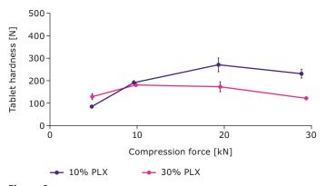
**Figure 6.**Tablet hardness after direct compression when using 10% and 30% Parteck® PLX 188 excipient.
