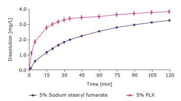
**Figure 9.**Comparison of the lubricant's effect on the dissolution profile of a sample itraconazole formulation.
