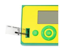
Make sure that no test strip is inserted in the test strip adapter, then press [OK].
