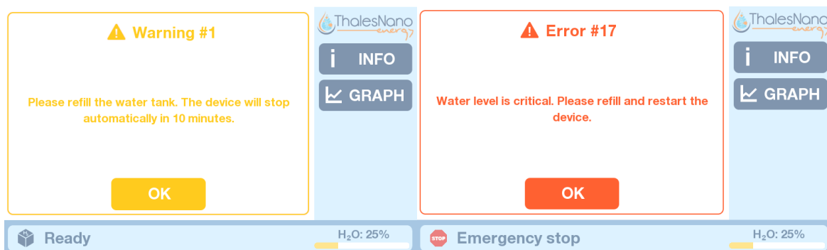
Figure 13: Warning and Emergency stop low water tank messages
