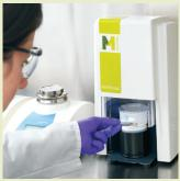
Put the unit into the MilliSnap™ system and close the safety glass
