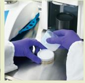
Take the unit out of the MilliSnap™ system and remove the funnel
