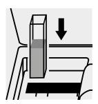
Place the cell into the cell compartment.
