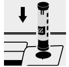
Select method with AutoSelector measuring range 10 – 250 mg/l Cl.
