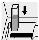
Place the cell into the cell compartment.
