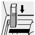
Place the cell into the cell compartment.
