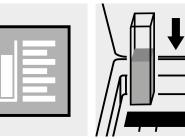
Place the cell into the cell compartment.
