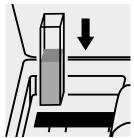
Place the cell into the cell compartment.
