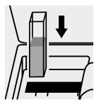
Place the cell into the cell compartment.
