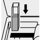
Place the cell into the cell compartment.
