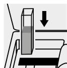
Place the cell into the cell compartment.
