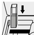
Place the cell into the cell compartment.
