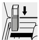
Place the cell into the cell compartment.
