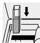
Place the cell into the cell compartment.
