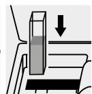
Place the cell into the cell compartment.
