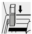
Place the cell into the cell compartment.
