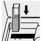
Place the cell into the cell compartment.
