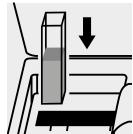
Place the cell into the cell compartment.
