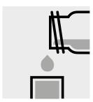
Transfer the solution into a rectangular cell.
