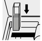
Place the cell into the cell compartment.
