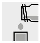
Transfer the solution into a 50-mm cell.
