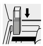
Place the cell into the cell compartment.
