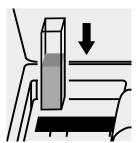
Place the cell into the cell compartment.
