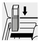
Place the cell into the cell compartment.
