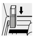
Place the cell into the cell compartment.
