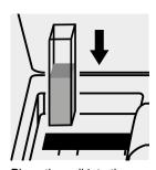
Place the cell into the cell compartment.
