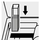
Place the cell into the cell compartment.
