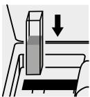
Place the cell into the cell compartment.
