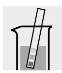
Check the pH of the sample, specified range: pH 3 – 8.
