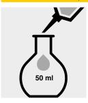
Place 1 ml of pretreated sample into a 50-ml volumetric flask.
