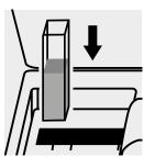
Place the cell into the cell compartment.
