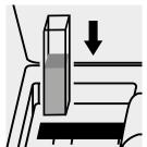
Place the cell into the cell compartment.
