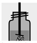
Disintegrate the filter in the homogenizer.
