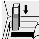
Place the cell into the cell compartment.
