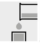
Transfer the **extraction** solution (reagent blank) into the cell.
