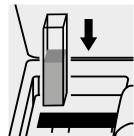
Place the cell into the cell compartment.
