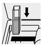
Place the cell into the cell compartment.
