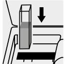
Place the cell into the cell compartment.
