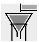
If contaminations are present, filter the sample over a fast filtering paper.
