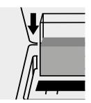
Place the cell into the cell compartment.
