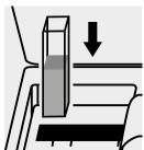
Place the cell into the cell compartment.
