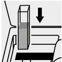
Place the cell into the cell compartment.
