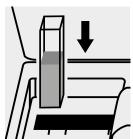
Place the cell into the cell compartment.
