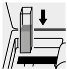
Place the cell into the cell compartment.
