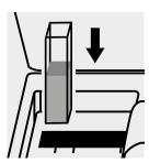
Place the **cell A** into the cell compartment. The measurement is performed automatically.
