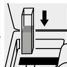
Place the cell into the cell compartment.
