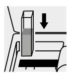
Place the cell into the cell compartment.
