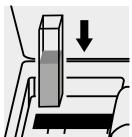
Place the cell into the cell compartment.
