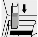
Place the cell into the cell compartment.
