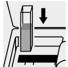
Place the cell into the cell compartment.
