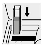
Place the cell into the cell compartment.
