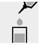
Transfer the solution into the quartz cell.
