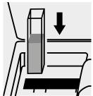
Place the cell into the cell compartment.
