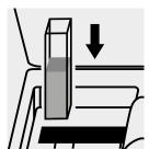
Place the cell into the cell compartment.
