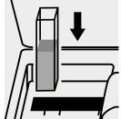
Place the cell into the cell compartment.
