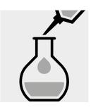
Make up the contents of the volumetric flask to the mark with cyclohexane for spectroscopy Uvasol® (Cat. No. 1.02822) and mix.
