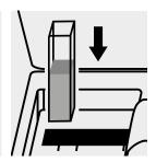
Place the cell into the cell compartment.
