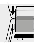
Place the cell into the cell compartment.
