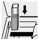
Place the cell into the cell compartment.
