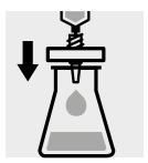
Filter or centrifuge turbid samples.
