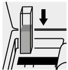
Place the cell into the cell compartment.
