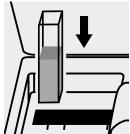
Place the cell into the cell compartment.
