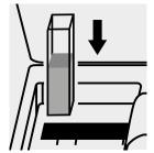
Place the cell into the cell compartment.
