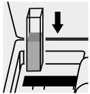
Place the cell into the cell compartment.
