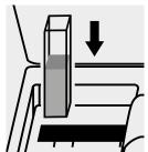
Place the cell into the cell compartment.
