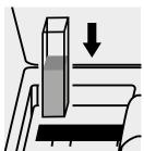
Place the cell into the cell compartment.
