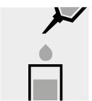
Transfer the solution into the quartz cell.
