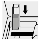
Place the cell into the cell compartment.
