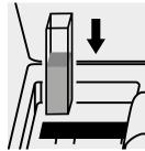
Place the cell into the cell compartment.
