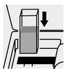
Place the cell into the cell compartment.
