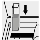
Place the cell into the cell compartment.
