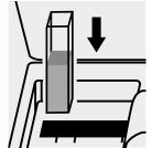
Place the cell into the cell compartment.
