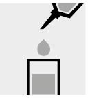
Transfer the solution into the quartz cell.
