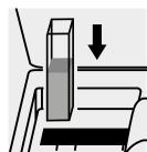
Place the cell into the cell compartment.
