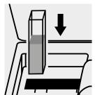
Place the cell into the cell compartment.
