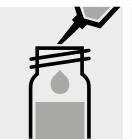
Carefully pipette 3.0 ml of the depleted blank tightly with the screw cap, cell, close tightly with the screw cap, and mix vigorously.
