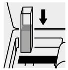
Place the cell into the cell compartment.
