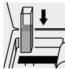
Place the cell into the cell compartment.
