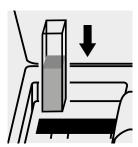
Place the cell into the cell compartment.
