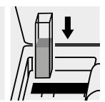
Place the cell into the cell compartment.
