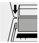
Place the cell into the cell compartment. The measurement is performed automatically.
