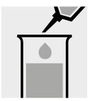
Pipette 5.0 ml of distilled Add to each tube 1.0 ml water (Water for analysis EMSURE®, Cat.No. 1.16754, is recommended) into a second test tube. (Blank)
