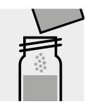
Add 1 powder pack of Molybdenum HR1, close with the screw cap, and dissolve the solid substance.
