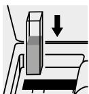
Place the cell into the cell compartment.
