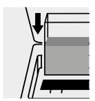
Place the cell into the cell compartment.
