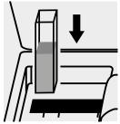
cell compartment. The measurement is performed automatically.
