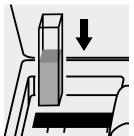
Place the cell into the cell compartment.
