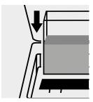
Place the cell into the cell compartment.
