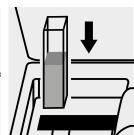
Place the cell into the cell compartment.
