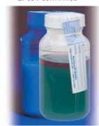
Just add a Readycult® Snap Pack to your sample and mix. Incubate up to 24 hours at 34.5°-37°C. If there is no color change the test is negative. (Turbidity does not indicate a positive test). Any color change in the broth to blue-green, even if only at the upper section, confirms the presence of total coliforms.
