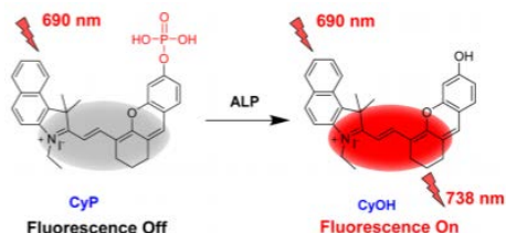
Figure 1. CyP AP mechanism. AP-catalyzed cleavage of the phosphate group in CyP AP induces the transformation of CyP into CyOH, which emits fluorescence in the near-infrared spectrum.
