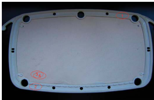
Figure 22. Location of spore strips inside Millistak+® Pod filter
