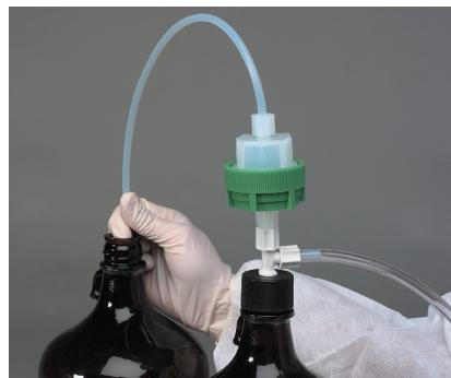
The HPLC Filter Degasser removes dissolved gas and particulates from Organic Solvents. It is designed to filter and degas 4 liters of solvent without operator attention at a rate of 4 liters per 10 minutes. The Filter Degasser uses a 0.2µm PTFE filter (sold separately) and is autoclavable at 120°C.
