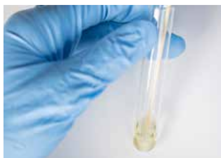
Transfer swab into 2 mL dilution broth (Letheen Broth) and vortex
