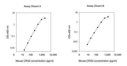
These standard curves are for demonstration only. A standard curve must be run with each assay.
