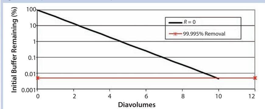
**Figure 2:** Percentage of initial buffer remaining and diavolumes; *R<sub>n</sub>* corresponds to run “*n*” as listed in Table 1.
