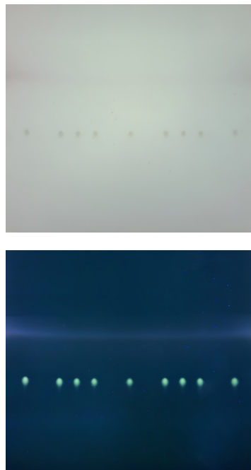
Figure 6. TLC Analysis of plate by the TLC Explorer under VIS excitation (top) and UV 366 nm excitation (bottom). The tracks 1, 5 and 9 are the dexamethasone sodium phosphate, reference and 2-4 and 6-8 are the samples. The plates were derivatized with a mixture of dihydroxybenzaldehyde, glacial acetic acid, and sulfuric acid.
