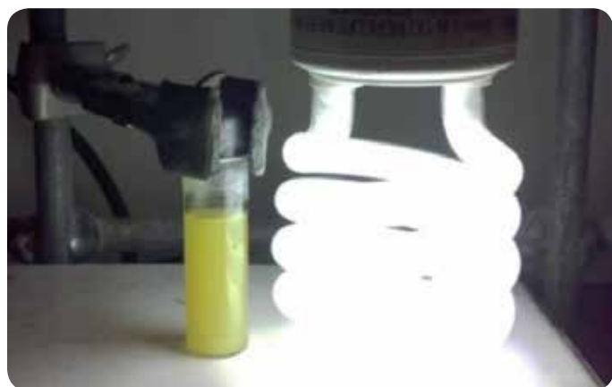
Figure 3. Photoreactor Setup With a 26 W CFL Lamp
