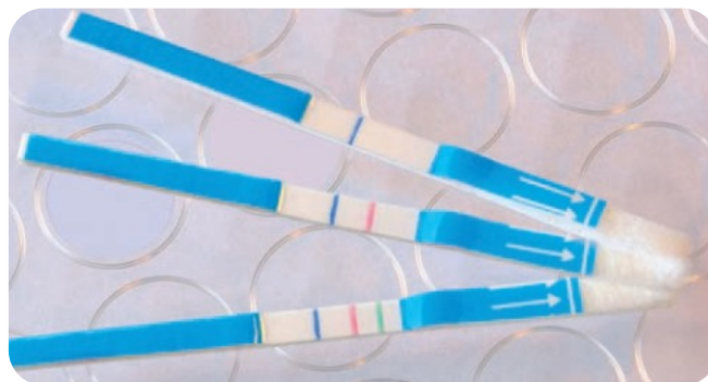
Lateral flow tests using Estapor® Dyed Microspheres (reference: K1-030 blue for the control, K1-030 red and K1-030 green for the analytes) and Millipore Hi-Flow™ membrane.
