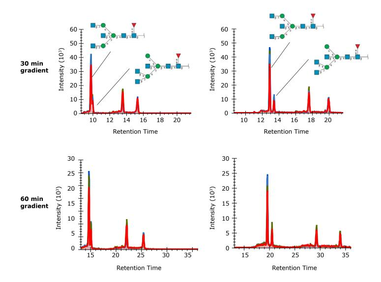
The above application illustrates the shape selective nature of PGC, and how not all PGC columns are similar. On PGC Column 1, even with a 60 minute gradient, two glycan isomers cannot be resolved, whereas on a Supel<sup>™</sup> Carbon LC column, a quicker 30 minute gradient enables baseline separation. Data courtesy of Dr. Christopher Ashwood, Beth Israel Deaconess Medical Center, Harvard University.
