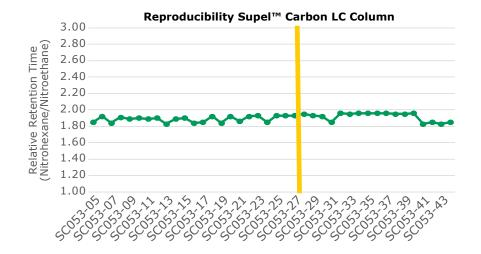
The capillary Supel<sup>™</sup> Carbon LC column demonstrates remarkable reproducibility between columns and lots. RRT relative standard deviation (RSD) was calculated to be only 2.4% between two lots of stationary phase, and the intercolumn RRT RSD was determined to be only 2.2% and 0.6% for lots 1 and 2, respectively. Yellow bar divides columns from Lot 1 and Lot 2.
