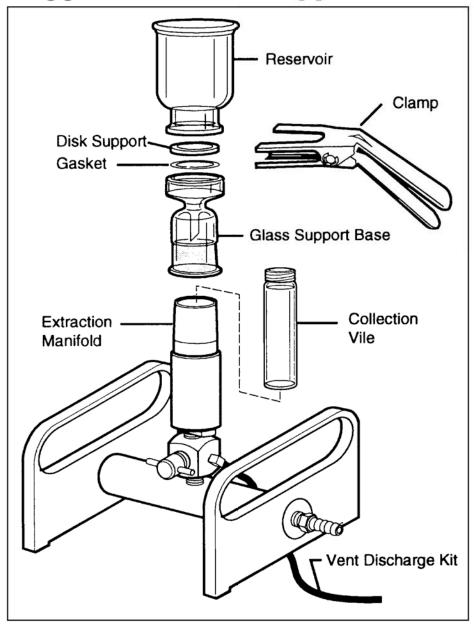
Note: Suggested solvent volumes will vary according to the disk diameter and the amount of Filter Aid 400 filter material. A general guide for solvent volumes is to completely cover the disk and bed of filter material, such that 2 - 3 mm of solvent is above the surface. Repeat with second aliquot.
